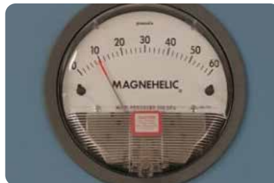
Magnehelic work chamber negative pressure gauge
